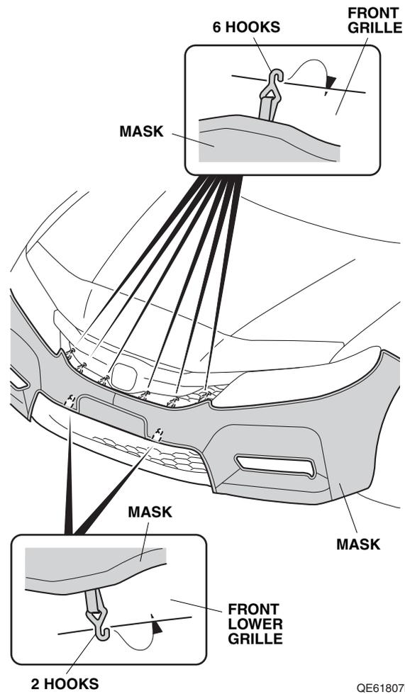
11. Attach two hooks to the inside edge of the front lower grille.
