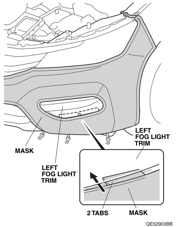
9. Pull the mask back toward the fenderwell, smooth out any wrinkles, and then snap the mask onto the snap-screw. Repeat on the right side.
