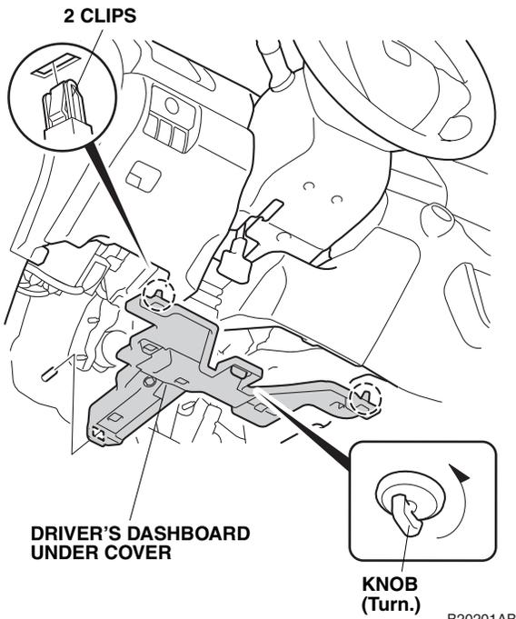
16. Remove the driver's dashboard lower cover and unplug the vehicle connectors, if equipped.
