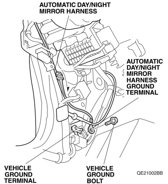
30. Remove the vehicle ground bolt. Secure the automatic day/night mirror harness ground terminal to the vehicle ground terminal, and reinstall the vehicle ground bolt.
