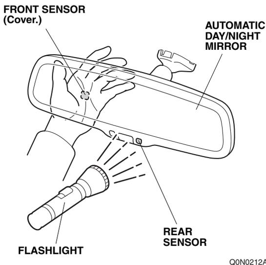
4. Step on the brake pedal, and move the select lever to the "R" position. Repeat step 3, and make sure the mirror surface does not dim.
