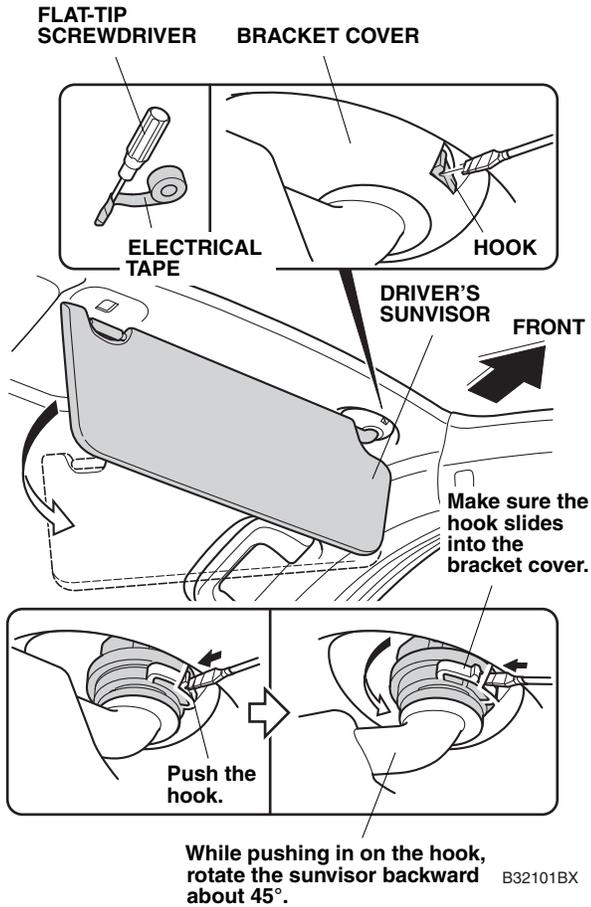
7. While pushing in on the hook, rotate the driver's sunvisor backward about 45°. Make sure the hook slides into the bracket cover.
