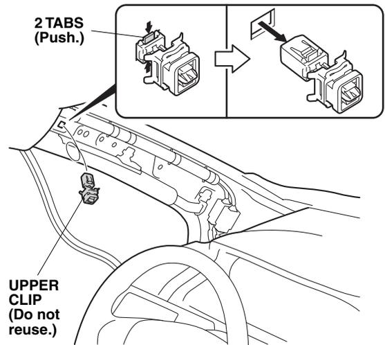
14. Install the new clip (supplied) on the driver's A-pillar trim, but do not reinstall the trim at this time.
