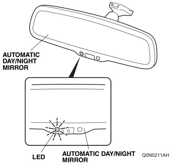
2. Turn on the switch. Check the LED lights.
