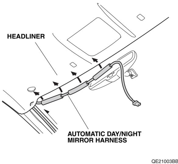
35. Secure the automatic day/night mirror harness to the vehicle harness with one wire tie. Make sure the automatic day/night mirror harness is not being stretched.
