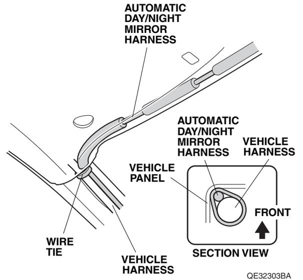
36. Plug the automatic day/night mirror harness 7-pin connector into the automatic day/night mirror.
