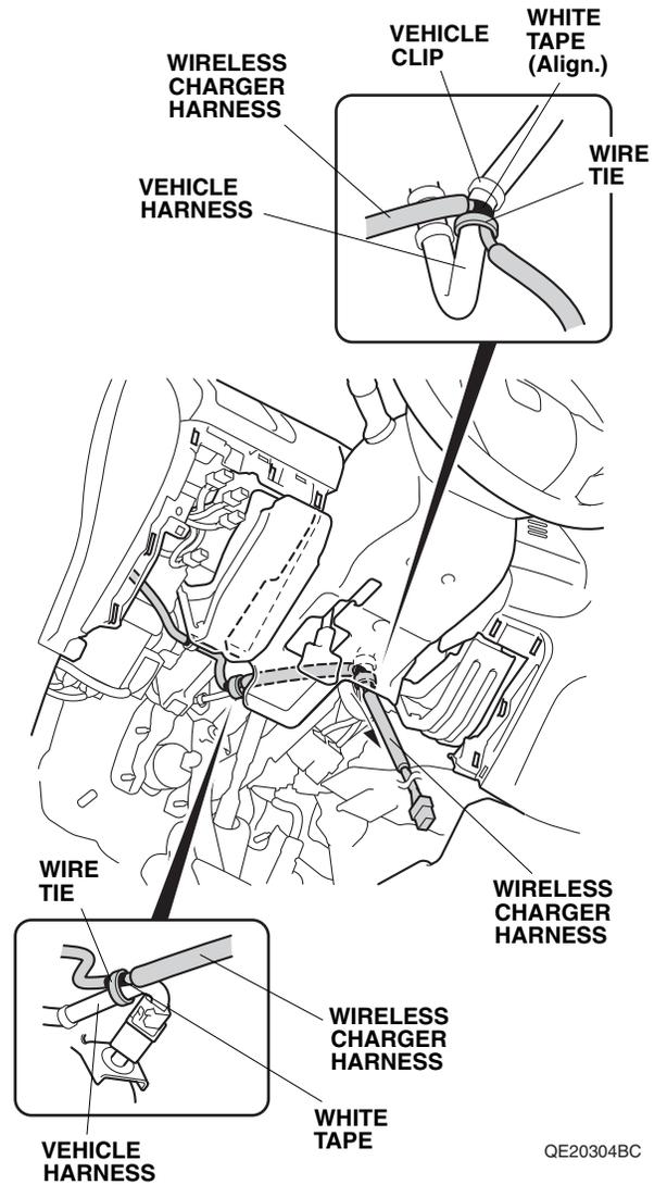
41. Secure the wireless charger harness to the vehicle harness with one wire tie at the white tape on the wireless charger harness.
