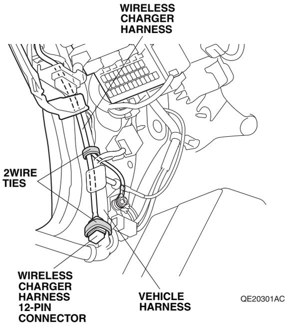
40. Align the white tape on the wireless charger harness with the vehicle clip and secure the wireless charger harness to the vehicle harness with one wire tie.
