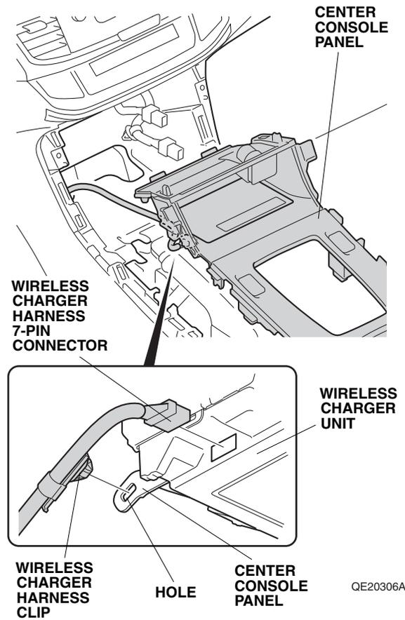
45. Secure the wireless charger harness to the center console panel with one clip on the wireless charger harness. Install the center console panel.
