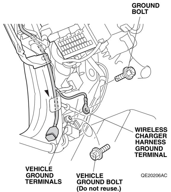
39. Secure the wireless charger harness 12-pin connector and wireless charger harness to the vehicle harness with two wire ties.
