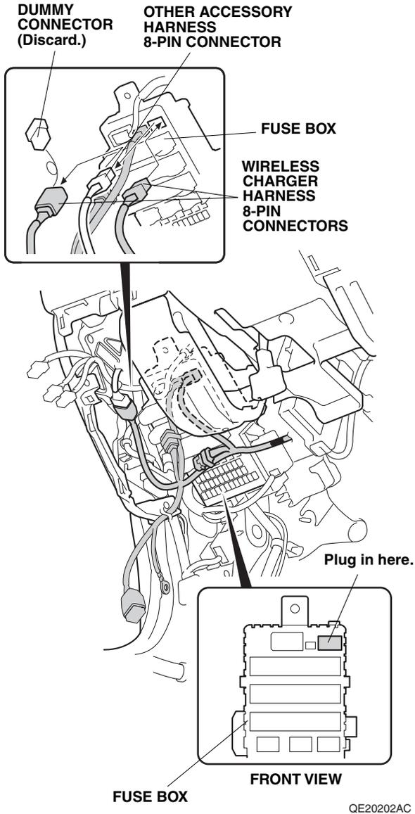
33. Plug the remaining wireless charger harness 8-pin connector into the fuse box.
