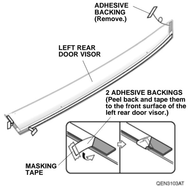
16. Remove the adhesive backing.
