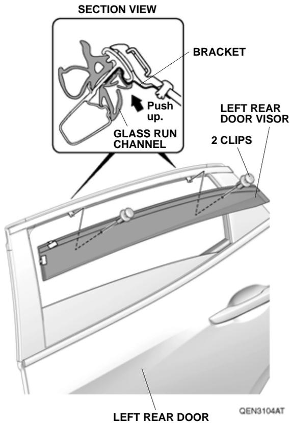
18. Secure the left rear door visor to the two brackets with the two clips. Make sure to push up on the brackets while installing the two clips. NOTE: Be extremely careful when installing the clips; they cannot be reinstalled after installation.
