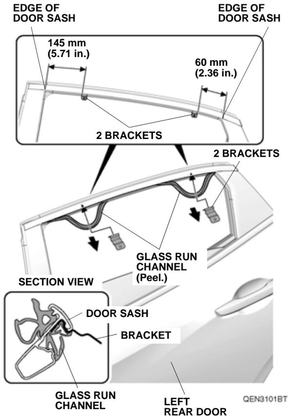
12. Peel the glass run channel as shown.
