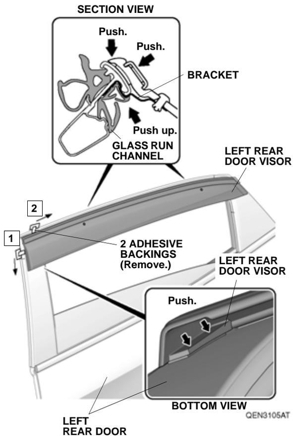
21. Using a soft towel, press and hold the left rear door visor against the door sash for 30 seconds.
