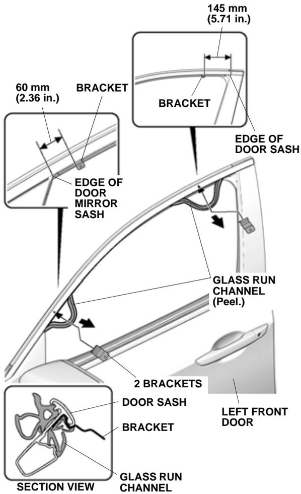
2. Peel the glass run channel as shown.
