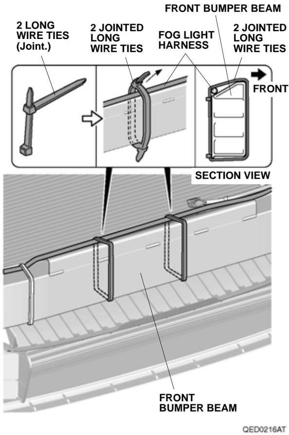
44. Secure the fog light harness to the vehicle harness with one wire tie.
