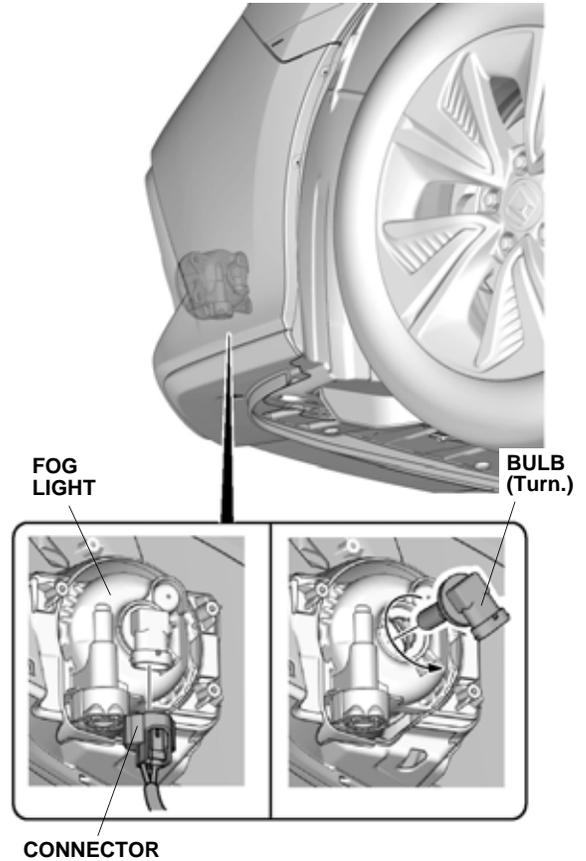
3. Remove the bulb from the fog light as shown.
