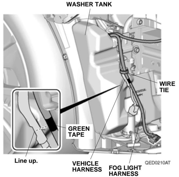
38. Secure the 1-pin connectors and fog light harness to the vehicle harness with three wire ties.
