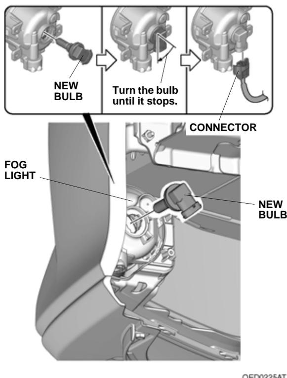
5. Install the removed parts. Check that the wire harness is not pinched and tighten the clips and bolt securely.
