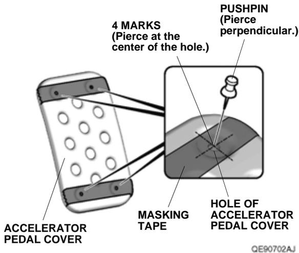
2. Using a pushpin, pierce masking tape as shown.
