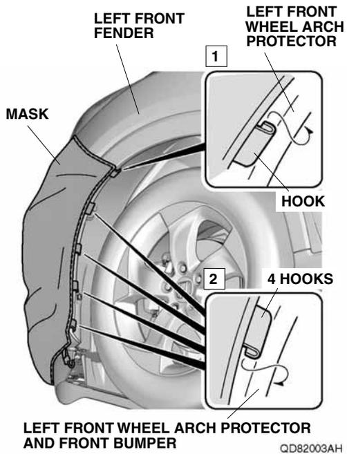
3. Attach four hooks on the mask's bumper section to the edge of the left front wheel arch protector and front bumper.
