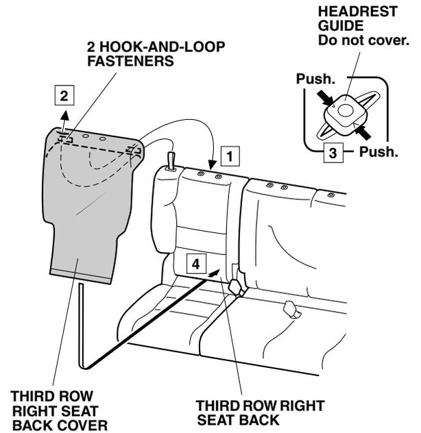
9. Fold down the third row right seat. Secure the third row right seat back cover to the third row right seat back with one hook-and-loop fastener. Return the third row right seat to the upright position.
