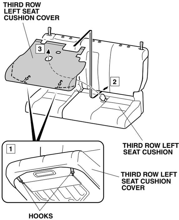
7. Secure the third row left seat cushion cover to the third row left seat cushion with the two hook-and-loop fasteners.
