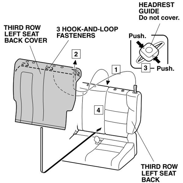
5. Fold down the third row left seat. Secure the third row left seat back cover to the third row left seat back with one hook-and-loop fastener. Return the third row left seat to the upright position.
