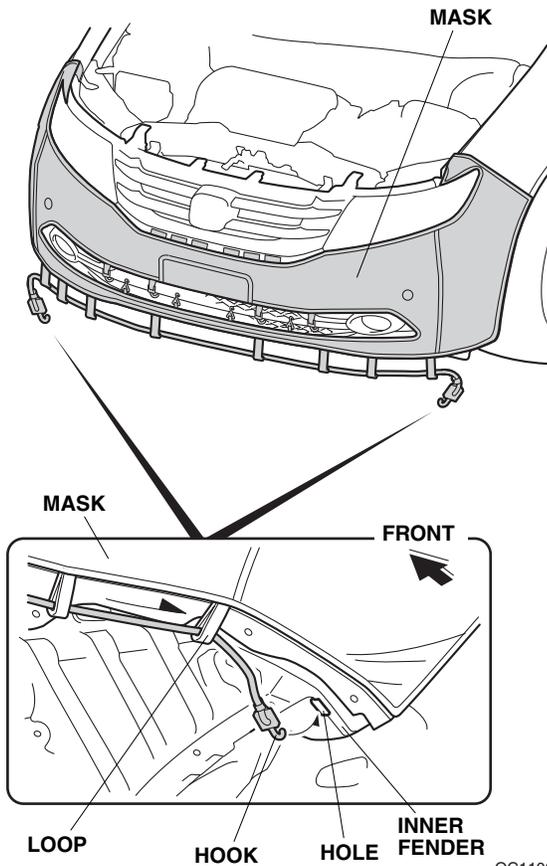
9. Secure one hook on the elastic cord to the hole of the inner fender.
