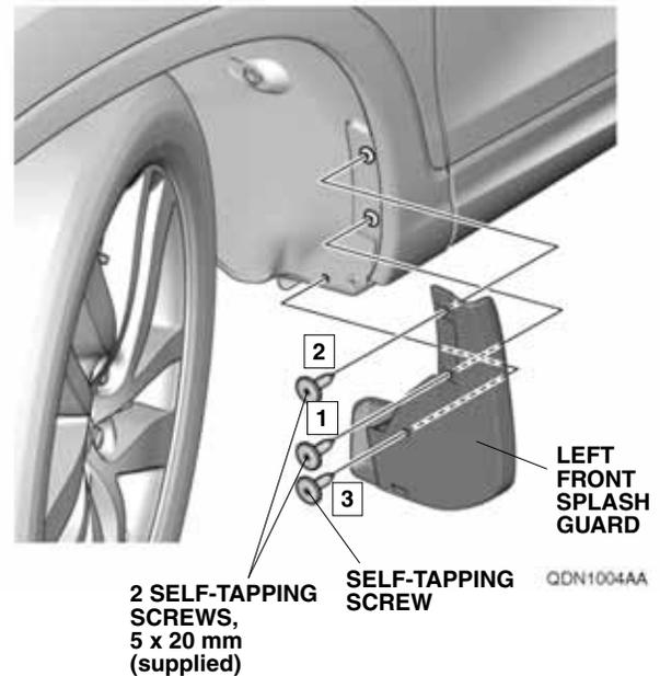
5. While holding the left front splash guard against the left front inner fender, tighten self-tapping screws in the order shown.
