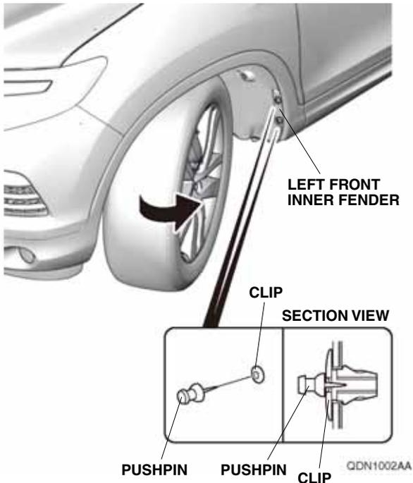
2. Using a pushpin, pierce the center of the top two clips on the left front inner fender.
