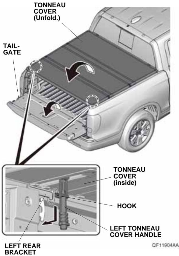
6. Pull down the left tonneau cover handle and slide outward while pulling down. Attach the hook to the left rear bracket. Repeat on the other side.
