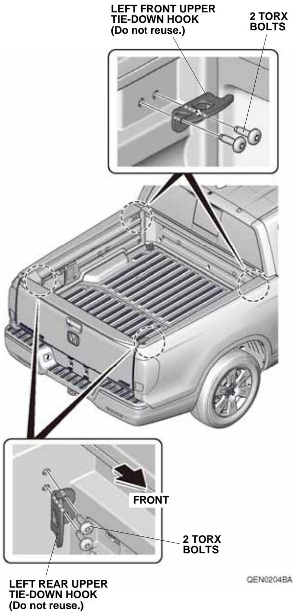
2. Install the left front bracket and left rear bracket to the left side bed lining with the four TORX bolts removed in step 1. Torque the TORX bolts to 20 N·m (15 lbf·ft). Repeat on the other side.
