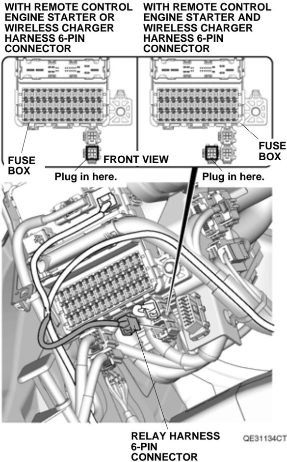
57. Secure the relay harness to the vehicle harness with five wire ties.
