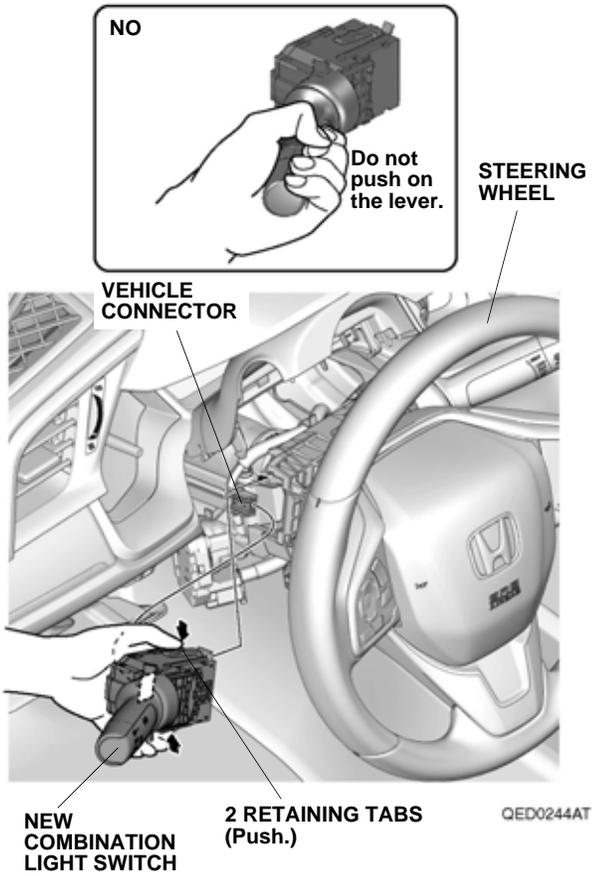
63. Plug the vehicle connector into the new combination light switch.
