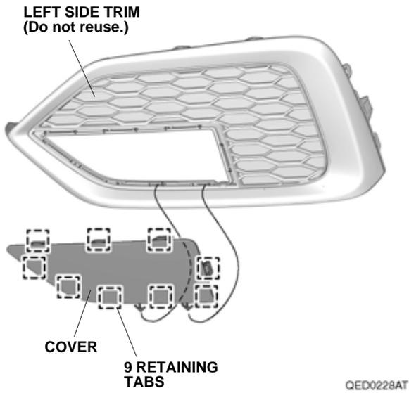
20. Install the cover to the left fog light trim with the nine retaining tabs.
