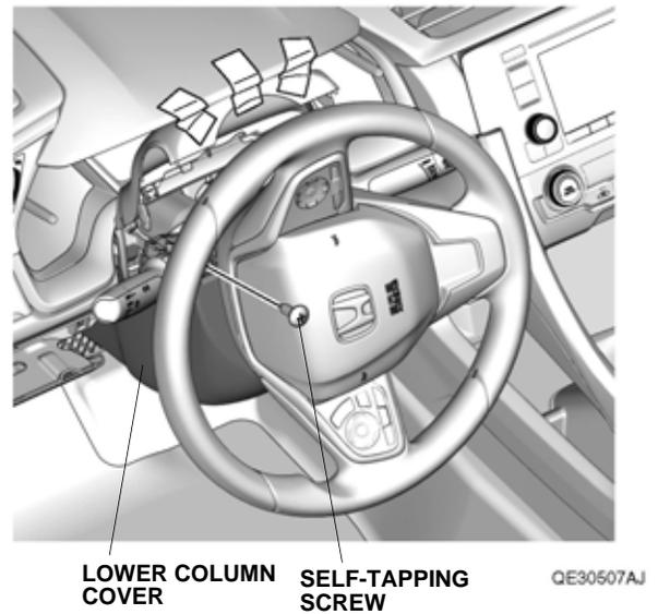
10. Turn the steering wheel 180° clockwise and remove the self-tapping screw from the lower column cover.
