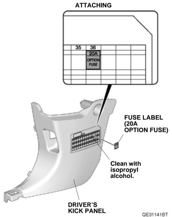
65. Attach the fuse label to the driver's kick panel.
