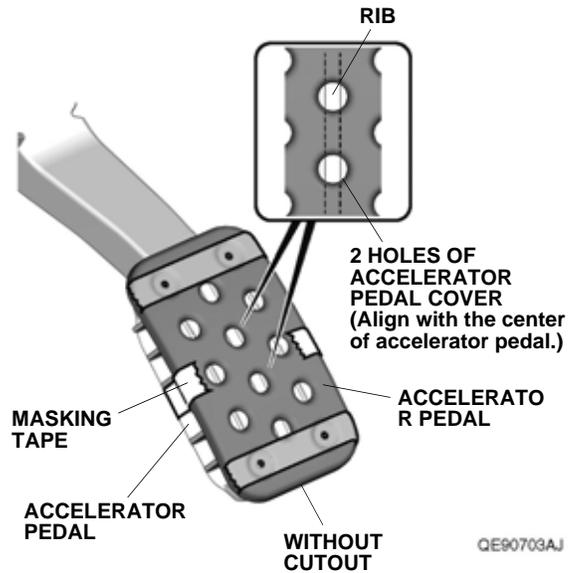
4. While wearing eye protection, drill the accelerator pedal at the four pierced marks with a 3.5mm drill bit.
