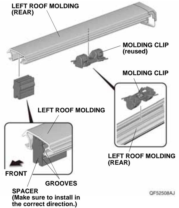
9. Install the left roof moldings back onto the roof of the vehicle as shown.
