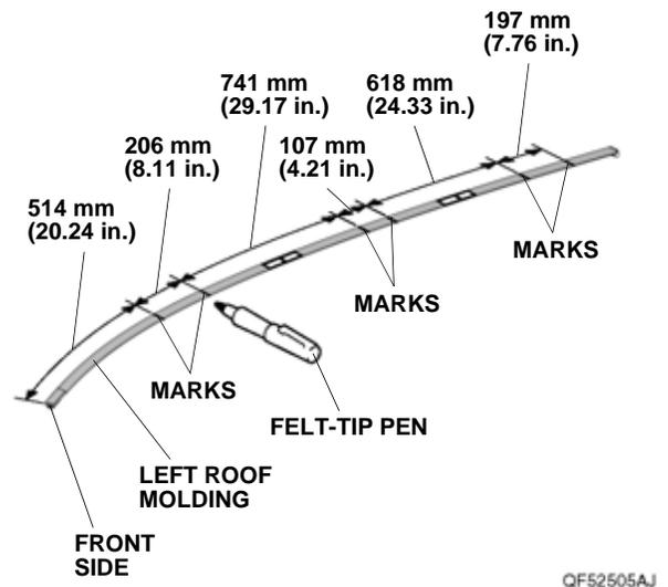
6. While wearing eye protection, use an air saw to cut the molding at the marks made in step 5. Remove any burrs.
